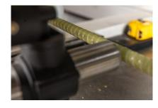
**GBar**® by COMPKING is a corrosion-free bar which aids in designing a structure with a much longer service life than traditional steel reinforced structures.
